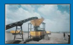
The mixed material from the pug mill is conveyed by the Load out conveyor and dropped into the storage silo. The silo is provided with hydraulically operated gate to retain processed material to minimized mixed material segregation during the load out cycle and spillage of mix product.
