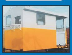
The Control Panel is housed inside an **insulated cabin**. The cabin is fabricated from M.S. sheet and is insulated. The cabin has glass windows all around, so that the **operator has full view** on all sides from the cabin for ease of operation and control.
